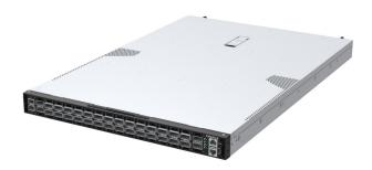
The DS4001 can support port level configuration of sub-rates between 10GbE and 400GbE. System maximum of 168 50GbE ports or 128 100GbE ports or 64 200GbE ports using breakout cables provides a superior fabric device for large radix CLOS networks. It provides superior low latency and power efficiency in a clean PHYless design, while offering high-reliability features such as redundant and hot swappable power supplies and fans.
